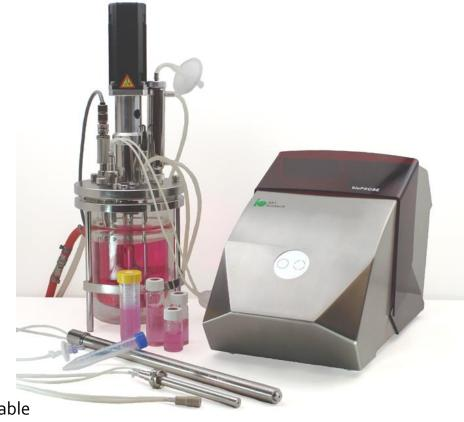
Sterile by design: no filters in the bioreactor, no issues with biofilms / biofouling, no influence on cultivation process
