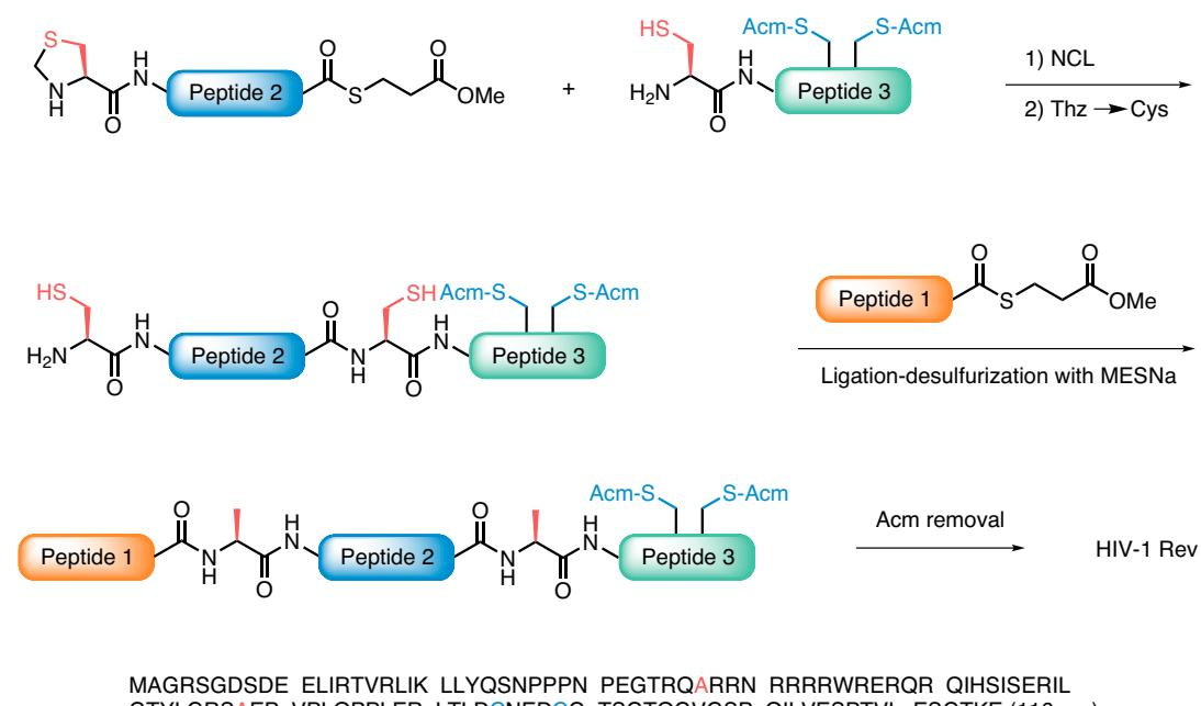
Fig. 16: Example of a synthesis of a peptide via ligation of three segments and thiazolidine as temporarily protected cysteine.
