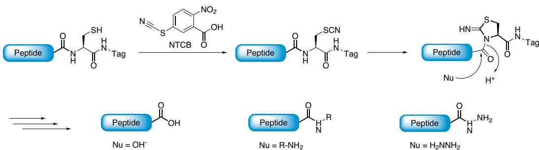
Fig. 13: Schematic illustration of the activated Cysteine-based protein ligation.
