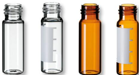
Standard sample vial of clear or amber glass with wide opening. 4 ml volume, thread 13-425. Borosilicate glass of the 1st hydrolytic class.
