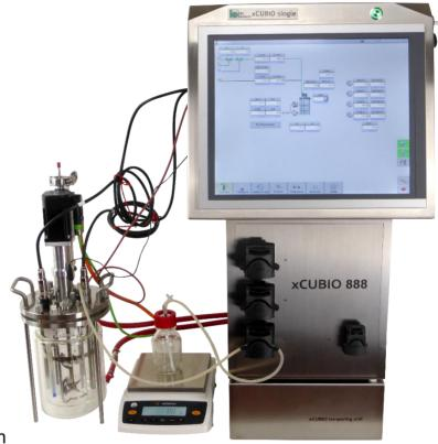
Integration of latest analysis technology like glucose control and automated bioprocess sampling
